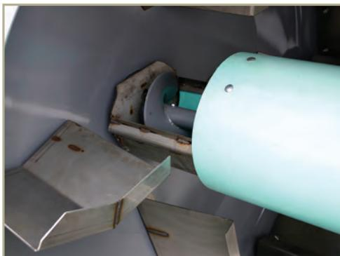
Balance in the mixing process is accomplished in a simple, effective manner. A sliding cover on the end of the auger allows more or less forage to enter the auger.
