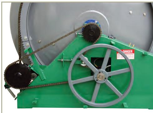
A super strong, quiet synthetic idler for the main drive chain is fully adjustable, while the drum drive utilizes a spring-loaded idler. All bearings have grease fittings for maintenance.
