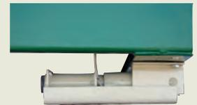
A weigh bar (one of four) mounts under the unit at each corner. Adds 4 3/4" to overall height.
